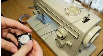
c. Wind the Clock Spring onto the Going Barrell by turning the Dial Hub clockwise when viewed from the front (in the above photo it would be counterclockwise).
