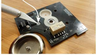
5. Lubricate and place the **Reduction** Gear (bag B). Place 2 Brass Washers on top of this gear.
