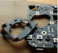
3. Place the Fingerstop (bag C) on the Dial Hub (bag A) as shown to check the fit. The Fingerstop should rotate on the Dial Hub without the hooked part of the Fingerstop scraping along the Dial Hub. If it does, the Fingerstop's hook may need to be re-shaped a bit with a needle-nose pliers, or there may be a bump on the Dial Hub, which can be smoothed down with a few strokes of an emery board.
