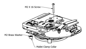
6. Rotate the Mallet Clamp Collar so that the notch is as shown.
