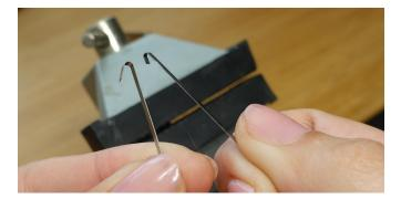
a. Hook the smaller hooked end of the Clock Spring onto the catch on the Going Barrell, and the larger hooked end onto the boss feature on the Front Bearing Pad.
