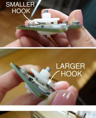
With both ends of the Clock Spring hooked to their respective catches, the extending loop of spring can be placed over a protrusion of some kind.
