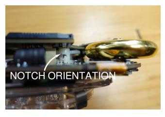
7. Install the **Mallet Assembly** into the slot formed between the Mallet Clamp Collar and Flange Bearing Pad, allowing the chamfered edge on the Mallet Spring to help guide it into the slot.
