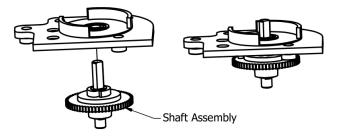
Press the Dial Hub (bag A) onto the protruding Dial Shaft, using the Bell Arm (bag C) as a shim to create a gap between the Dial Hub and the bearing.
