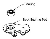
2. Glue the Back Bearing Pad onto the **Daughterboard** on the same side as the SIM and microSD card holders.
