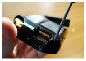
15. Maneuver the Bell Window (bag A) into place by wedging the casing open as necessary. The tabs on the Bell Window will retain it in the enclosure.
