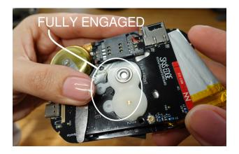
8. Test the rotary mechanism. Generally, it will feel stiff at first and may bind. Exercise it; Subtle burrs need to get worn off the newly made gears, and the lubricant needs to be spread throughout the mechanism.
