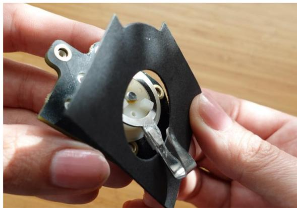
13. Slip the Dial **Face Window** (bag F) over the Fingerstop and into place, aligning roughly as shown.
