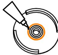
4. Glue the **Front Bearing Pad** into the **Faceplate** on the side opposite the PEM nuts.
