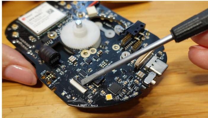
2. Remove the protective film from the **OLED Display** (bag D) and insert it between the Motherboard and Faceboard, roughly aligned with the white markings on the Motherboard.
