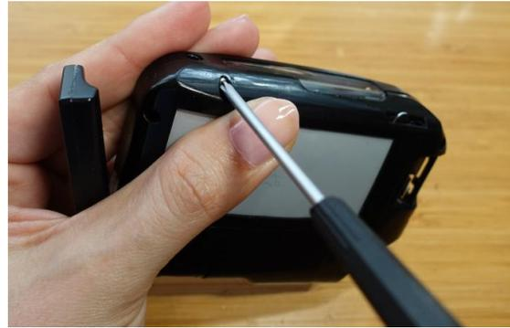
13. The Side Window has a tendency to unseat during assembly. With the phone oriented with this window facing down (for gravitational assistance), a sharp object can be inserted through the nearby seam to nudge it into position.
