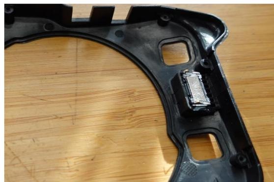
7. With the Back Enclosure/electronics assembly sitting face up, set the **Side Window** (bag E) into the Back Enclosure.
