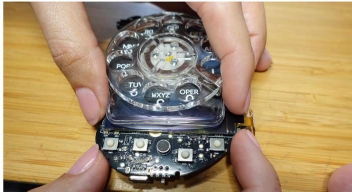
3. Wrap the OLED Display's flex cable around the motherboard edge and insert it into the connector on the Motherboard.
