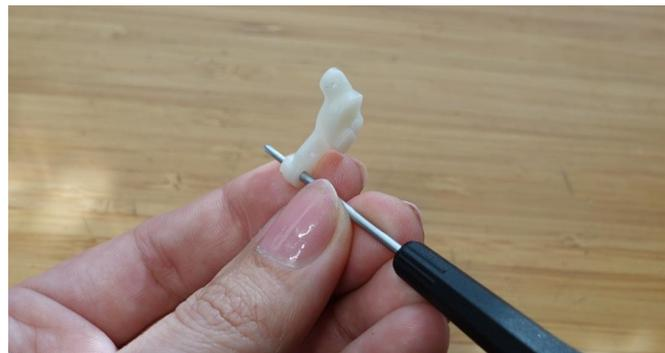
20. Screw the Flange Bearing Pad onto the Motherboard using two **M1.6X4 Screws** as shown.
