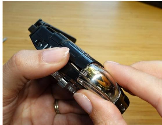
16. Insert a **M1.6 X 8 Self Threading Screw** into the hole under the SIM opening.
