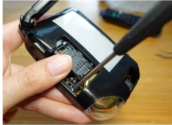
17. Tighten **M1.6 X 6 Self Threading Screws** into the remaining empty holes.
