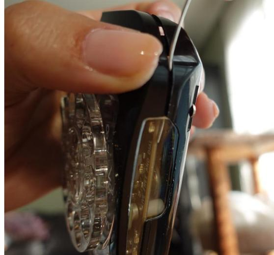
14. Tighten an **M1.6 X 6 Self Threading Screw** into the hole nearest the volume slot to secure.
