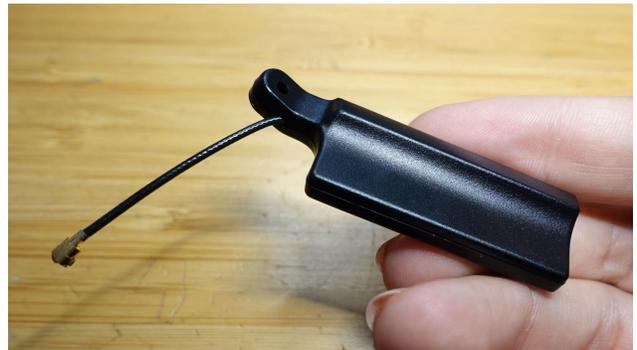
Add a healthy gob of hot glue over the antenna board and near the perimeter, then briskly squeeze the **Outer Antenna Enclosure** onto the Inner Antenna Enclosure until dry.
