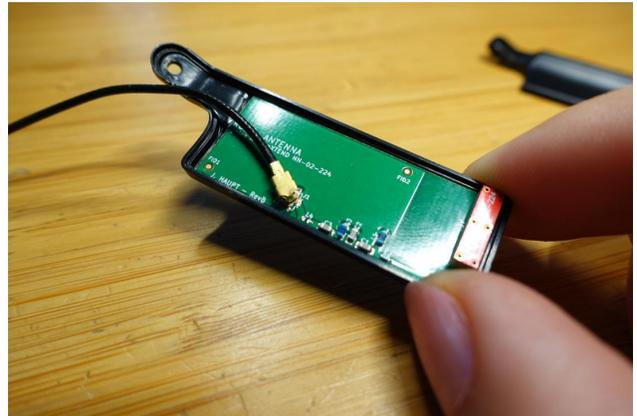
3. When the **Outer Antenna Enclosure** (bag E) is installed over the Inner Antenna Enclosure, the cable exits through a cutout near the hinge feature. Test-fit the two enclosure halves together to confirm proper cable routing, and then separate them again.
