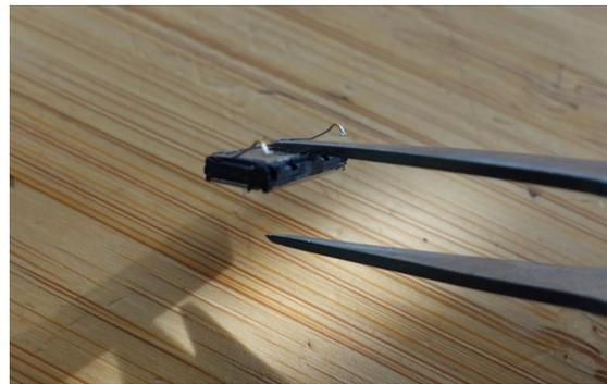
6. Press the Speaker into the speaker grill on the **Front Enclosure** (bag E). The hooked part of the speaker's contacts should face toward the center of the phone.
