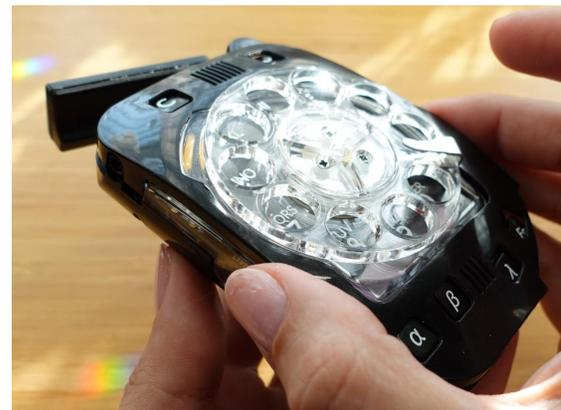
10. Gently wiggle and jostle it until the internal components set and the enclosure halves can be firmly squeezed together.
