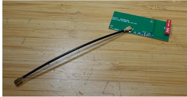
2. Hot glue the Antenna Board into the **Inner Antenna Enclosure** (bag E).
