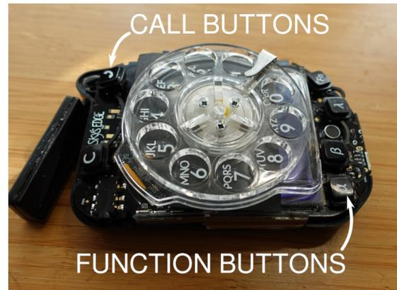
9. Set the Front Enclosure over the whole phone, tweaking the buttons into place as you compress the halves together.
