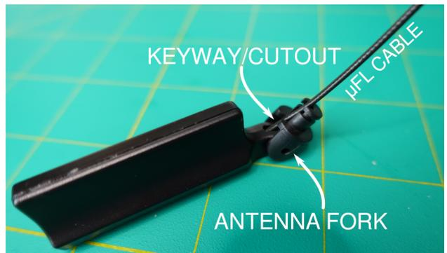
5. With a mallet, tap the **M2X10 Dowel** through the Antenna Fork and Antenna Assembly, capturing the Antenna Fork onto the Antenna Assembly.
