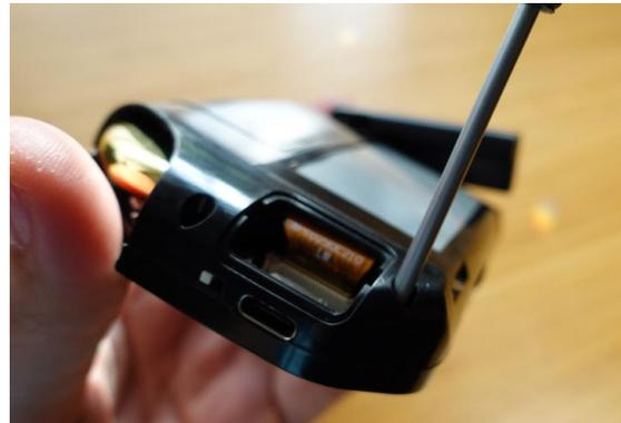
15. Maneuver the **Bell Window** (bag E) into place by wedging the casing open as necessary. The tabs on the Bell Window will retain it in the enclosure.
