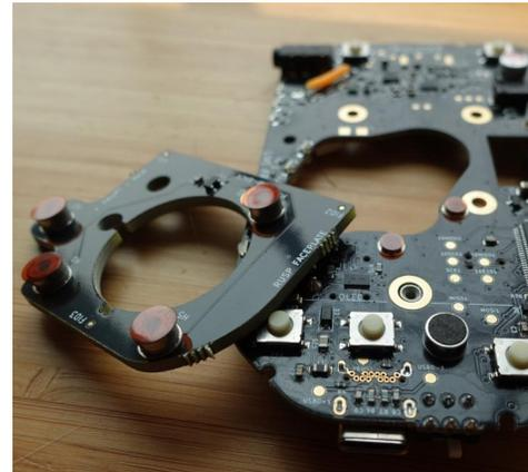
3. Place the **Fingerstop** (bag C) on the **Dial Hub** (bag E) as shown to check the fit. The Fingerstop should rotate on the Dial Hub without the hooked part of the Fingerstop scraping along the Dial Hub. If it does, the Fingerstop's hook may need to be re-shaped a bit with a needle-nose pliers, or there may be a bump on the Dial Hub, which can be smoothed down with a few strokes of an emery board.
